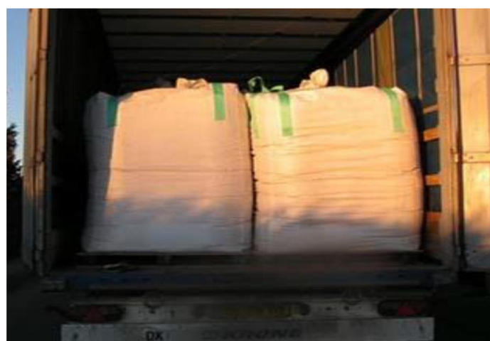
Figure 11: Concentrate transported in 1m 3 bulk bags
